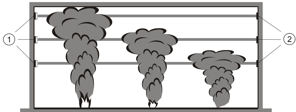
Detection of smoldering fires in high rooms on different levels
